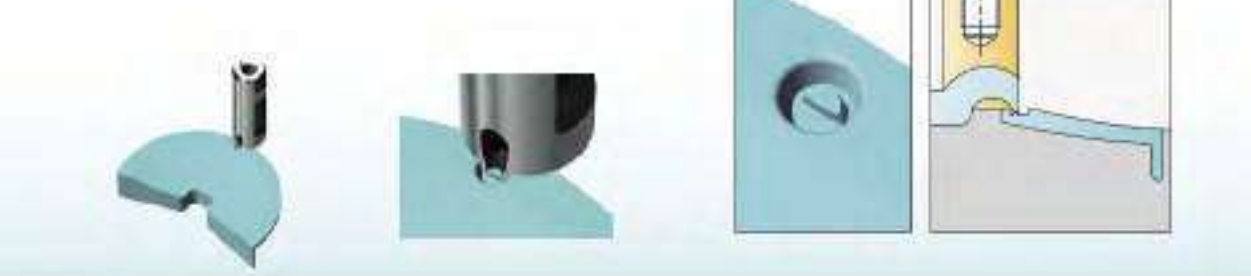
flat part with companion vestige - installation in fixed half of the mold
