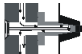
Conventional core cooling using a brass baffle.
