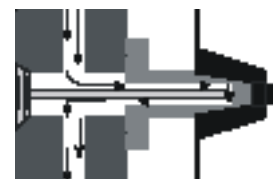
Conventional core cooling using a brass baffle.
