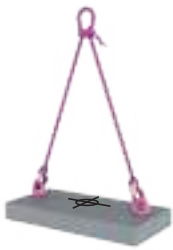
Symmetrical load Central centre of gravity
