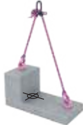
Asymmetrical load Centre of gravity off-centre
