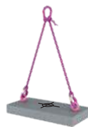
Symmetrical load: Central centre of gravity
