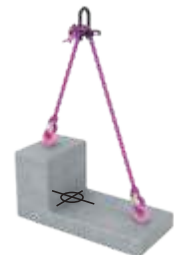
Asymmetrical load: Centre of gravity off-centre
