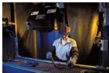
Magnaflux Crack Detection
