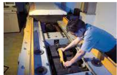
Tensile Test, Capacity 300 tonnes
