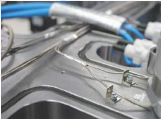
Hot runner bar with steel tube and mounting bracket
