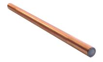
Cooling Pins are high speed heat transfer devices capable of conducting heat energy over 10,000 times faster than copper, thus cooling molds faster and reducing cycle time. Cooling Pins are used to heat or cool cores, slides and inserts in thermoset and thermoplastic molds. This isothermic device allows for optimal heat transfer rates within cores and slides.
