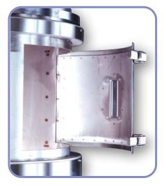
Laser-cut access doors provide a smooth, tight fit and eliminates troublesome gaskets
