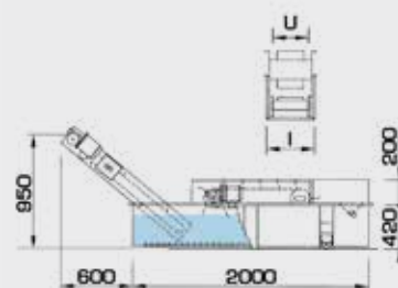
NV7 - NV8 - NV9 Nastro vasca particolari galleggianti e non galleggianti Conveyor with cooling tank for floating and no floating parts
