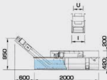
NV4 - NV5 - NV6 Nastro vasca particolari galleggianti Conveyor with cooling tank for floating parts
